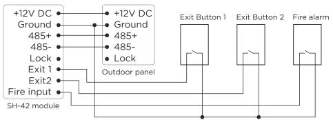
To connect the output control button of the first relay, use contacts **«Exit 1»** and **«GND»**, and to connect the control output button with the second relay, contacts **«Exit 2»** and **«GND»**. The **«Fire input»** and **«GND»** contacts are used to connect the fire alarm output contacts.
