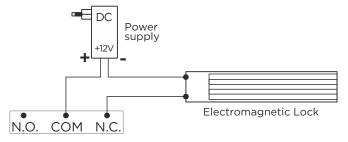
With such a connection in the power circuit of the lock, you must use the contacts: **COM** (switchable contact) and **N.C.** (normally closed contact).
