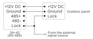
In this case, the module is connected to the call panel with three wires: +12 V power supply, Ground, and Lock. With this connection, it is possible to control only the first relay. When an external control signal module is applied to the «Lock» input, only the first relay will act on switching. For the «Lock» input, it is necessary to use a low-voltage external signal with a DC voltage from +9 to +12 V.
