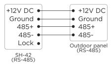
In this case, the call panel is connected to the module via four wires: + 12 V power supply, Ground, 485+ and 485-. With such a connection, it is possible to control two relays independently of each other.
