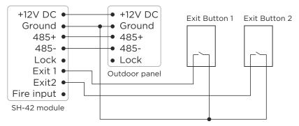
The exit button for controlling the first relay is connected to the **«Exit 1»** and **«GND»** contacts, and the exit button to control the second relay is connected to the **«Exit 2»** and **«GND»** contacts.
