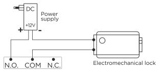
With such a connection in the power circuit of the lock, you must use the contacts: **COM** (switchable contact) and **N.O.** (normally open contact).
