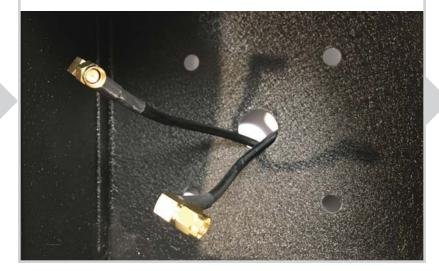
9 Attach antenna assembly to antenna pole and connect 25' antenna cables.
