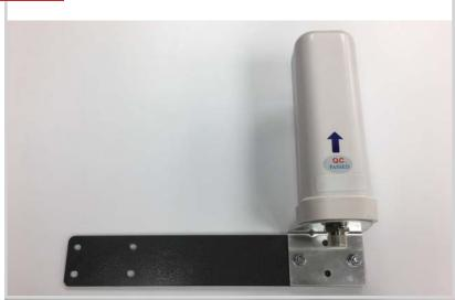
Overlap mounting brackets to prepare for U-bolt installation.
