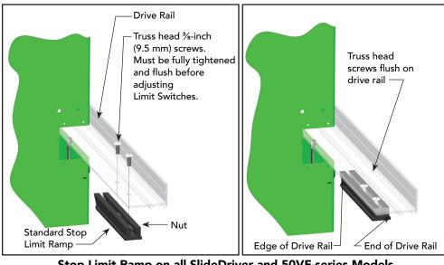
Stop Limit Ramp on all SlideDriver and 50VF-series Models
