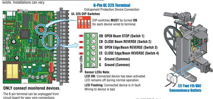
Type of wiring to be used on ALL external devices: A) Type CL2, CL2P, CL2R, or CL2X.
