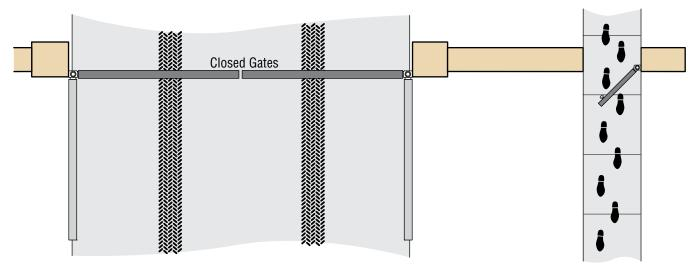
Entrapment Protection must be provided for the gate system where the risk of entrapment or obstruction exists. The operator will NOT run without one or more monitored type B1 or B2 entrapment protection devices in EACH ENTRAPMENT AREA.
