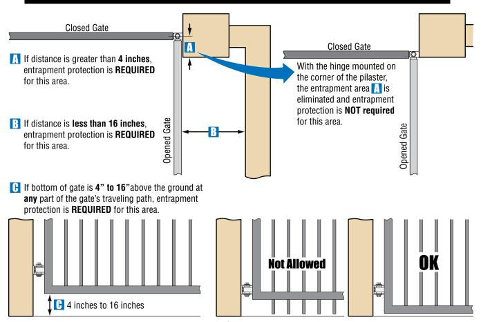
Gates shall have smooth bottom edges, with vertical bottom edged protrusions **NOT** exceeding **0.50** inches.
