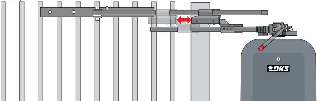
Mark and cut off excess arms. Secure arms to elbow assembly with 6 allen screws. Tighten hub and replace release tool. Install
