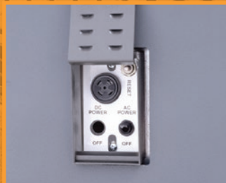
Built In power switch and reset switch
