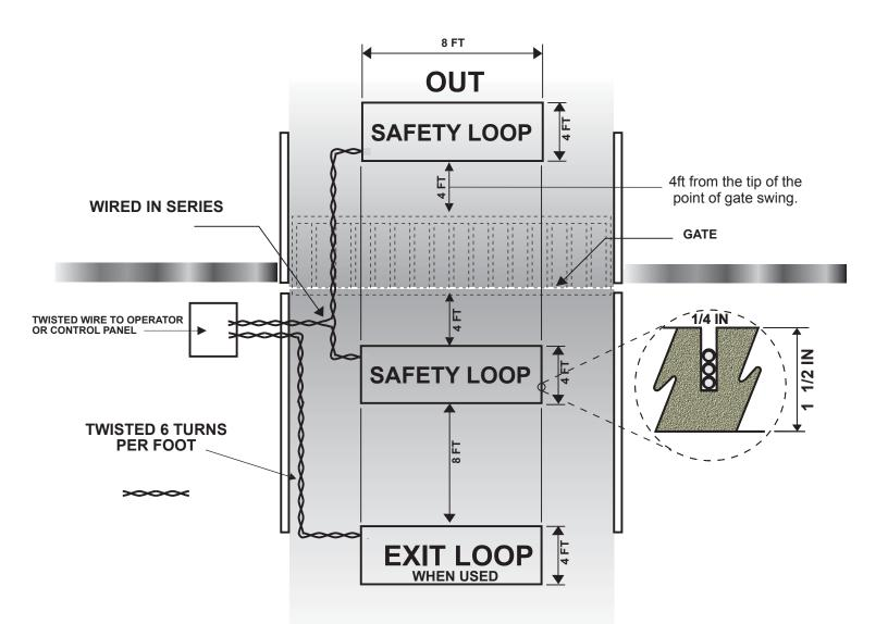
This is a normal loop layout. Remember when connecting to an All-O-Matic circuit board you use the **normally closed contacts** for your safety loop detector and **normally open contacts** from the exit loop. You must twist your wires from your exit point of the saw cut all the way to the circuit board, no exceptions.
