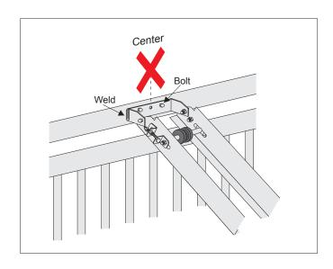
Make sure end bracket is in the center of the opening. Bolt or weld the end bracket to wall. The operator bracket must be at least 2.5" above the gate.
