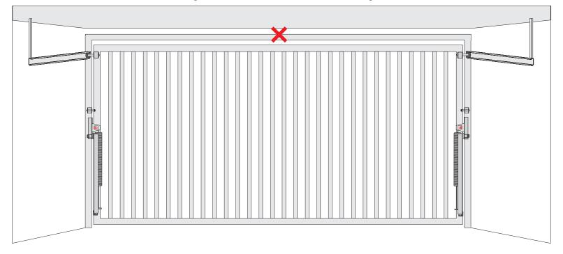
Lift gate to open position and mark the center point of the gate for the operator on the ceiling.
