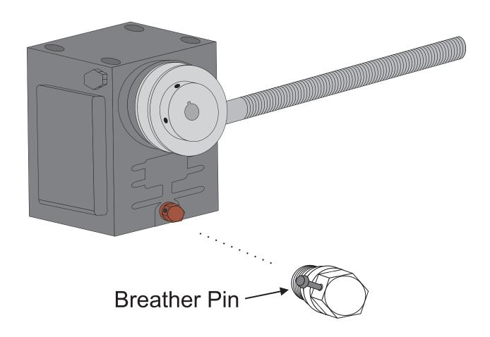
After installation remove breather cap pin for proper operation.
