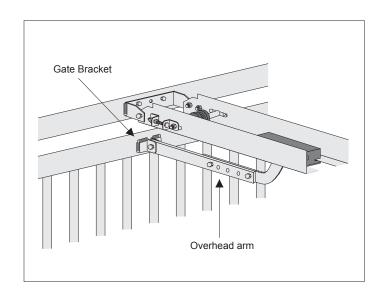
Weld gate bracket into place with overhead arm connected to insure alignment.
