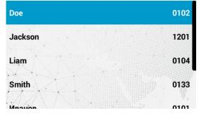
Press «\*» to exit the main screen or it will be done automatically, after 30 sec of inactivity.
