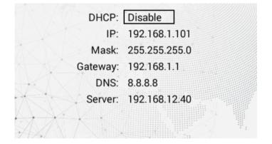
Here you can turn on/off **DHCP** connection and get network settings automatically or enter it manually.
