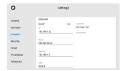
By default, a device can have a static IP address of 192.168.1.90 or 192.168.1.91.
