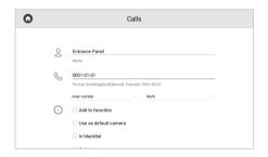
An inner number of a multi-apartment panel consists of Building No., Unit No., and Device No. For example, 0001-01-1 is the number of the panel located in the 1st unit of building No. 1.
