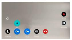
• **Call down** mode stands for only down moving. Users can call the elevator from the monitor (to the floor where the monitor is installed) or from the Link app (to the floor where the apartment is) with the help of a down calling button. 16 ports are available for downward movement.
