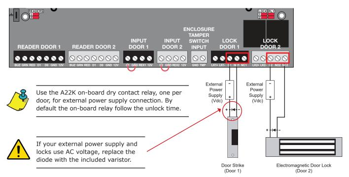
See "Recommended Wiring" section for more information on wiring type, size, and maximum length.
