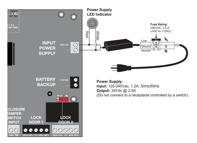
See "Recommended Wiring" section for more information on wiring type, size, and maximum length.
