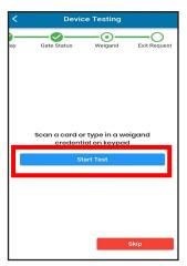
2. Verify that the Wiegand information you entered displays. An incorrect or blank code generally indicates a wiring problem.
