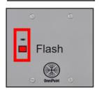
A red flash indicates that the device has **no** connection to the gateway.
