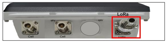
Once the lightning controller is attached, you can install the antenna. The antenna attaches to the lightning controller, so the device is protected form potential lightning strike.
