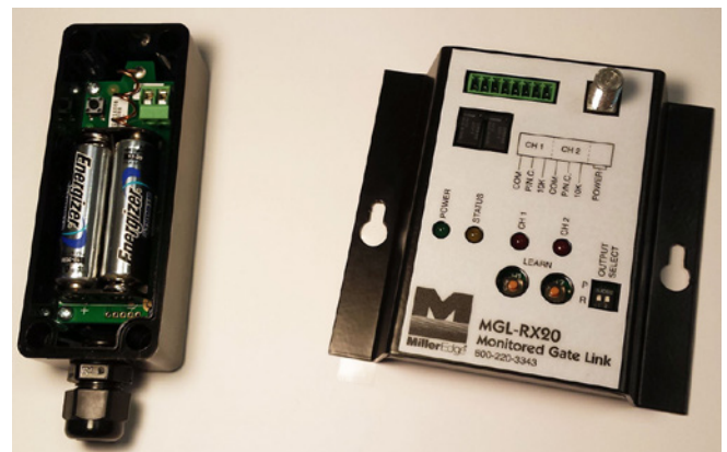
Example: Wireless gate link (transmitter & receiver) used with wireless gate edges
