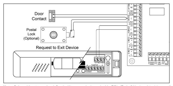
**Note:** Onboard inputs can be defined with: none, single or double EOL (End-of-Line) resistor(s) according to your settings with the VUI or with EntraPass.
