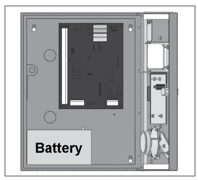
*Note:* The battery must be kept indoor if the outdoor temperature drops below -25°C (-13°F).
