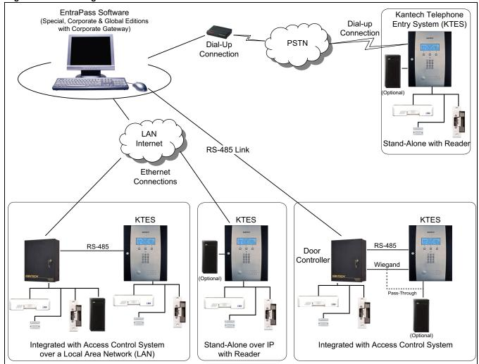
**Note:** For the UL 294 Compliance, the KTES-US and KTES-CDN models must be integrated with an access control system over a Wiegand connection.
