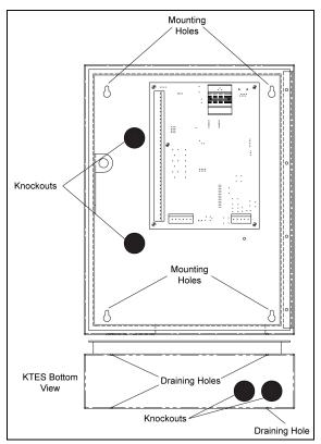
**Figure 11: Surface Mount Installation** Top View of KTES Surface Mounted 3.17 cm (1 1/4 in) (1 1/4 in) 22.86 cm (9 in) 7.65 cm (3 in) 3.17 cm (1 1/4 in) 8 37.56 cm (14 3/4 in) 31.10 cm (12 1/4 in) 29.25 cm (11 1/2 in) 3.17 cm (1 1/4 in) 7.65 cm (3 in) 22.86 cm 3.17 cm 3.17 cm (9 in) (1 1/4 in) (1 1/4 in) 3.80 cm 2.54 cm (1 in) (1 1/2 in)
