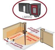
If the distance between the open gate and the wall is less than 16" (40.6 cm) entrapment protection for this area is required. Entrapment protection is required for the area between the gate and the curb.
