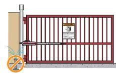
DO NOT install next to sprinklers or any area that may expose the bottom of operator to water.
