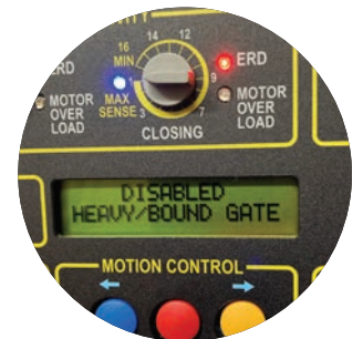
Heavy gate or binding gate detected
