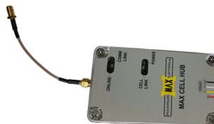
c. Place Max Cell Hub inside the Control Box and secure it with velcro
