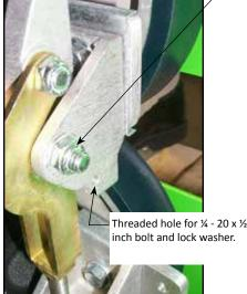
Remove the lock nut, but leave the pivot bolt in place.
