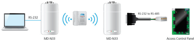
Figure 21: Remote Site Modem Configuration
