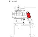
Viking ECU Use extension cable to bring Antenna outside of the metal casing
