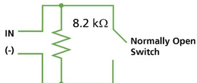
Normally Open Supervised inputs with one resistor must be connected with an 8.2K resistor in parallel to the input switch contacts.
