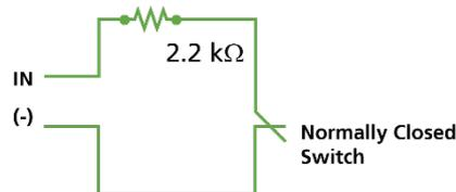
Normally Closed Supervised inputs with a single resistor must be connected with a 2.2K resistor in series to the input switch contacts.
