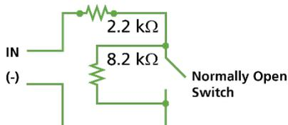
Normally Open Supervised inputs with two resistors must be connected with an 8.2K resistor in parallel and a 2.2K resistor in series to the input switch contacts.
