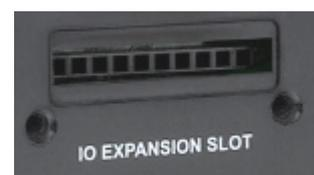
The text on the MD-D02B must face the same way as the text on the panel cover.
